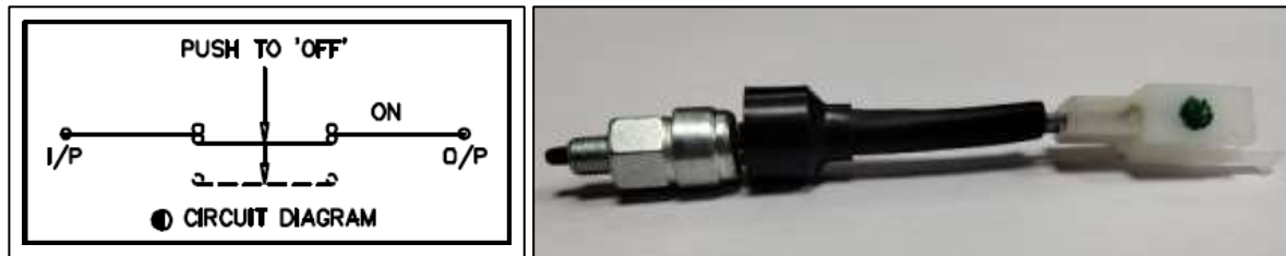
Figure 12 Clutch Switch with Circuit Diagram
