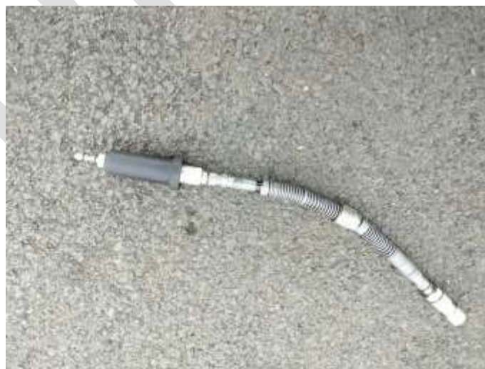
CNG Gas Filling Nozzle
