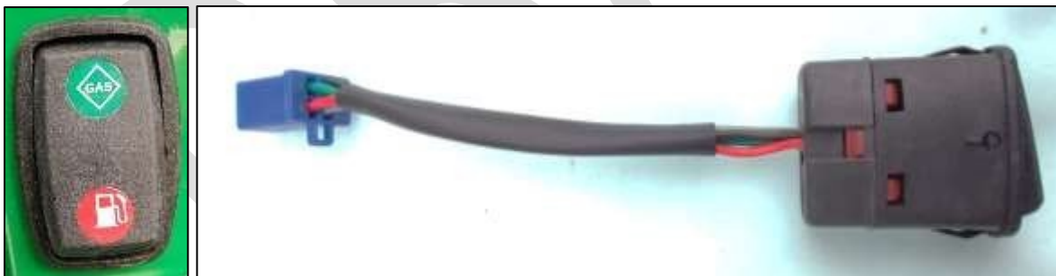
Figure 9 Fuel Mode Selector Switch
