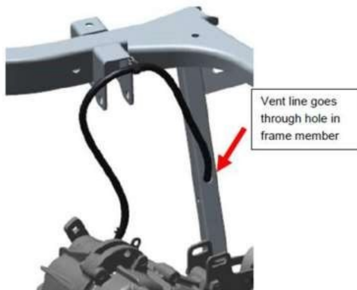
Figure B- 57: Example of a gearbox vent tube terminating inside a frame member.
