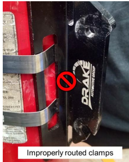
Figure B-52: Incorrect routing of hose clamps.
