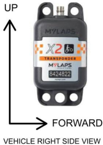
Figure B-66: Transponder Orientation
